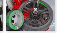
The tire changer dual rollers hold the tire in place to match the stiffest point on the tire to the lowest point on the rim.
