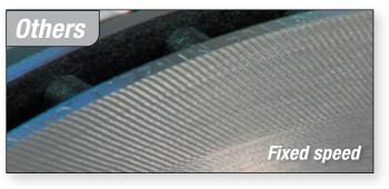
Chatter can start when machining rotors at a fixed speed. This is similar to a how a moistened finger can make a crystal glass sing.
