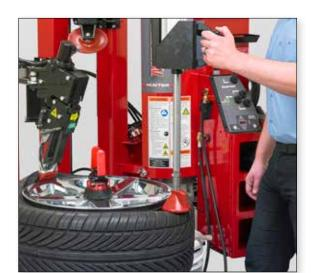
✓ Bead ledge allows pusher to be used as a lifting device also
