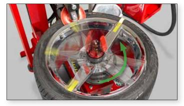
The Maverick<sup>™</sup> tire changer's bead rollers allow spinning of tire on rim, helping match-mount stiffest point on tire to low spot on rim.
